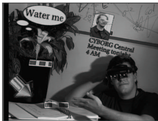
Figure 2: Multiple graphical overlays aligned through visual tag tracking. The color code in each tag provides a unique ID for the object. In addition, the vision process tracks each tag in 2.5D as the head-mounted camera moves.
